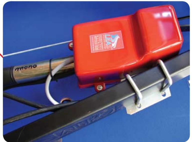
the trailer. As soon as the trailer becomes unstable (i.e. snaking occurs) the electronic control unit gives a signal to the actuating motor to release the spring and thus activate the braking system of the trailer (with 20% of its full braking performance). The car/trailer combination is stretched and reverts to a stable condition. The acoustic warning signal ensures that the driver knows that the braking system has been deployed by the LEAS unit.
